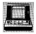
PEN SPEED: 1 second for full scale transverse. CHART TAKE-UP: automatic, by motor with preset torque-or by-pass for free end chart tear off.
